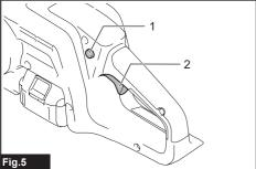
1. Lock-off button 2. Switch trigger
