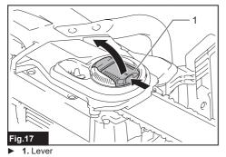
**2.** Turn the lever counterclockwise a little to loosen the sprocket cover lightly.
