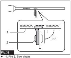
The file can be guided more easily if a file holder (optional accessory) is employed. The file holder has markings for the correct sharpening angle of 30° (align the markings parallel to the saw chain) and limits the depth of penetration (to 4/5 of the file diameter).
