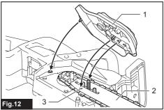
1. Sprocket cover 2. Guide bar 3. Hole
