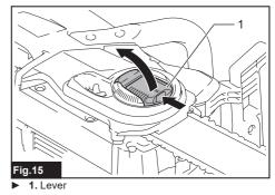
**4.** Turn the lever counterclockwise until the sprocket cover comes off.
